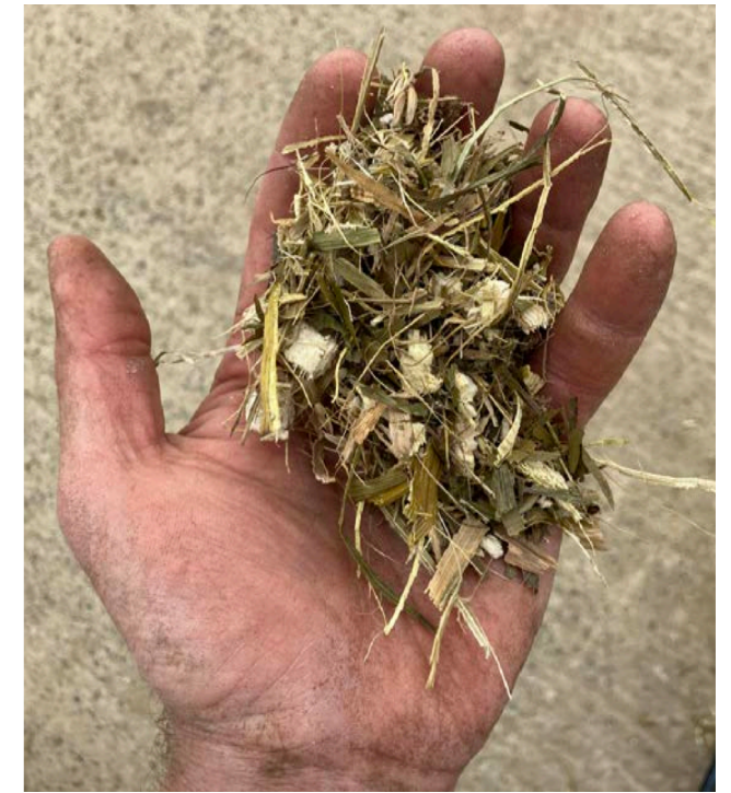
Dry shredded sweetcorn plant - note the varied particles - the pithy insulating core and longer leaf fibres
