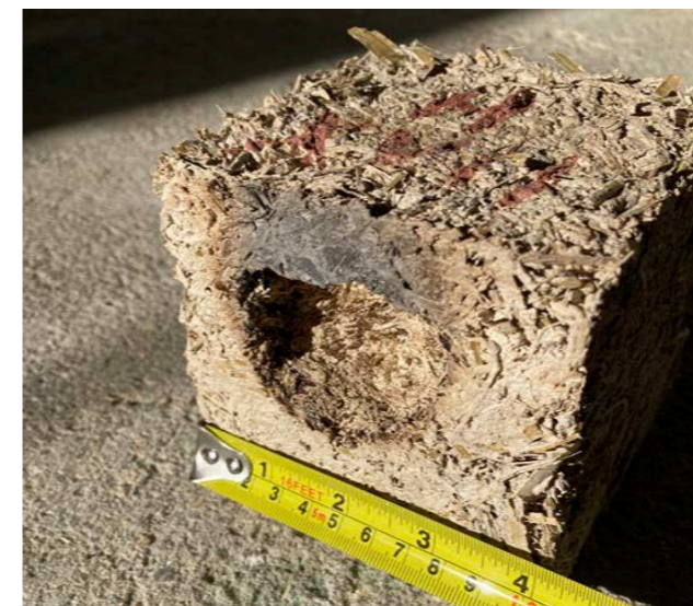
Damage to a sweetcorn block from a 90 minute fire test at 600C
