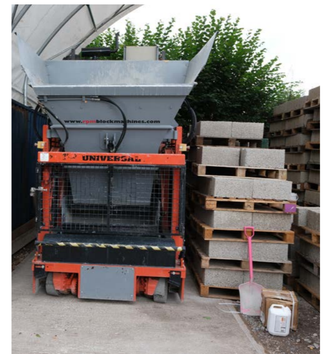
Adapted concrete block making machine currently used for hemp
