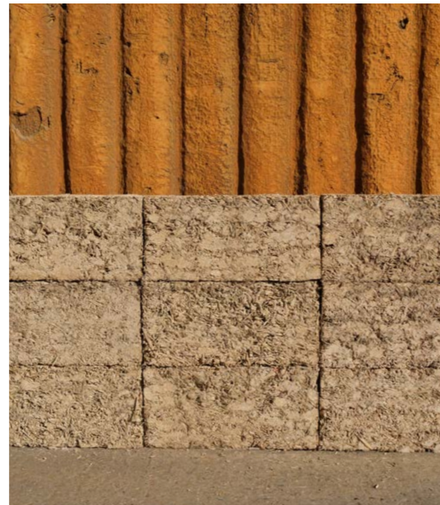
Prototype insulation blocks in cold-store barn next to expanding foam insulation, for comparison
